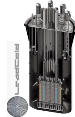
LeadCold SEALER 1-10 MWe, Sweden Under design
